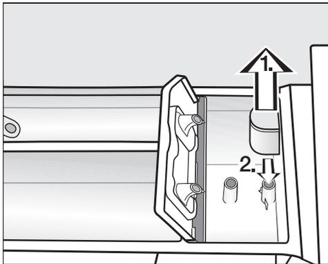
1. Remove the siphon from the
